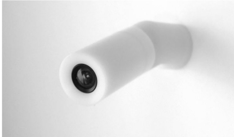
Figure 5.9: Wall mounted cylinder shaped camera with an adjustable joint.
