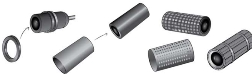
Figure 5.4: Concept 13, cylinder camera with exchangeable skins.
