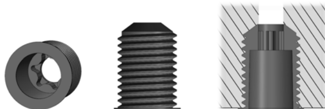
Figure 6.22: Mounting bracket 3, for recessed camera. M30 standardised threads with a small taper and a Torx screw patterned hole for installation with screwdriver.
