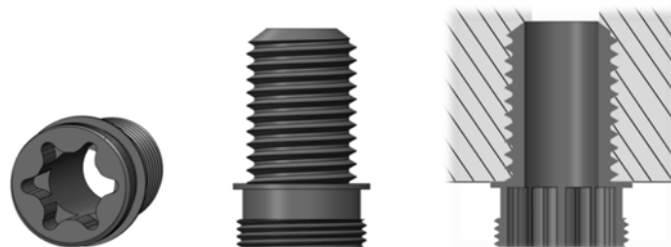
Figure 6.15: Mounting screw 3, for the adjustable camera. M20 standardised threads and a Torx screw patterned hole for installation with screwdriver.
