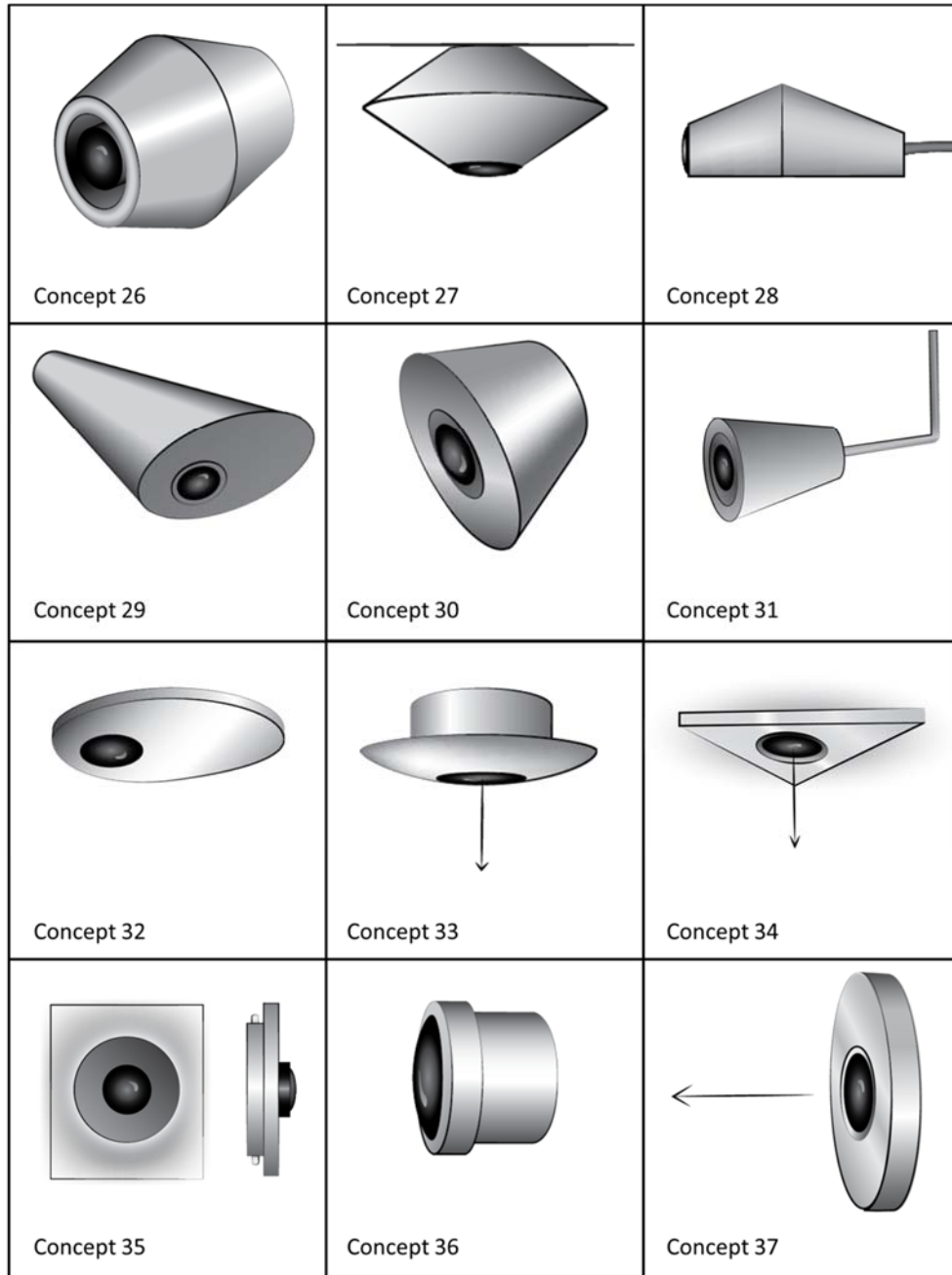
Figure 4.8: Generated concepts. 26 – 34: Shape variations. 35: Camera with background light - “halo”. 36 – 37: Shape variations.
