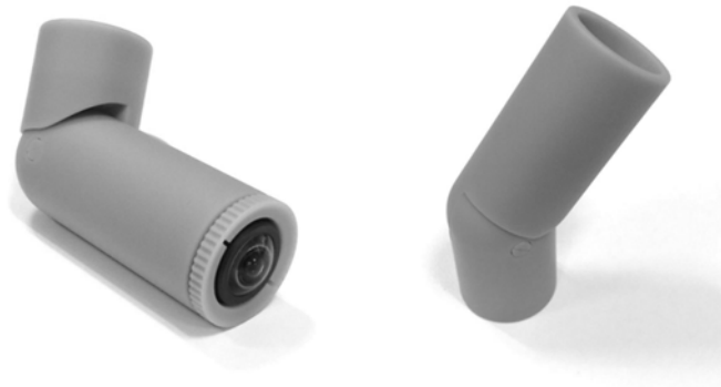
Figure 6.5: 3D printed models of the adjustable camera, containing the base unit on the left and detached on the right.
