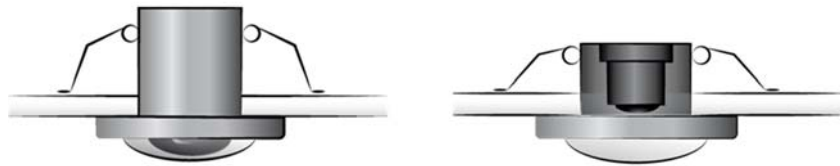
Figure 5.6: Concept 71, recessed camera with springs holding the mounting bracket. The recessed mounting solution is inspired by the AXIS M3011/M3014 camera, mentioned in chapter 4.5. The camera is partially hidden and can be very discreet.
