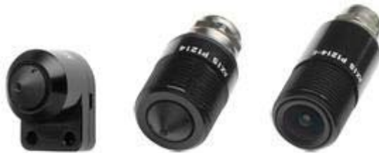
Figure 1.1: The sensor units in the AXIS P12 series. The camera to the left has the dimensions 27 x 20 x 22 mm (H x W x D). The two cameras to the right have a diameter of 20 mm and the longer version is developed for outdoor use [4] - [6].
