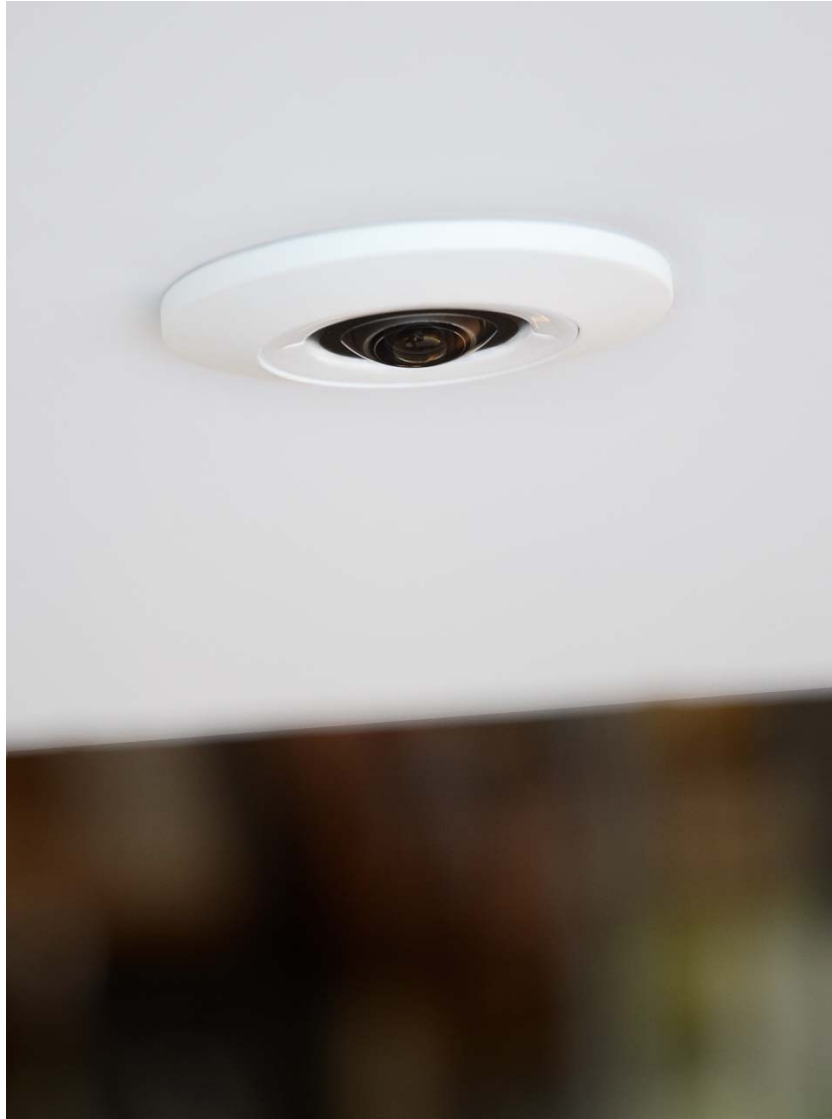
Figure 7.3: 3D-printed model of the recessed mounted camera placed in the ceiling.
