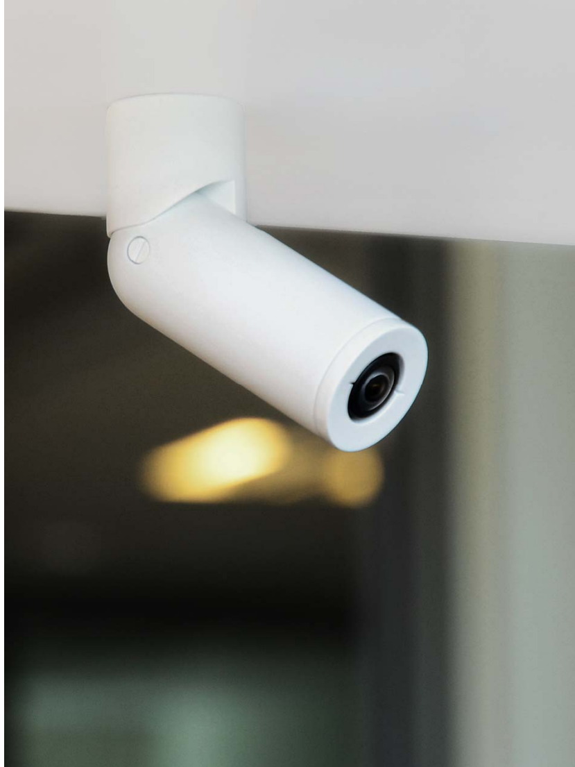
Figure 7.2: 3D-printed model of the adjustable camera placed in the ceiling.
