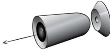
Figure 5.7: Concept 75, magnetic ball and socket joint. The magnetic ball and socket joint was one of the selected concepts due to its slenderness, ease of installation and its ability to conceal the cable.
