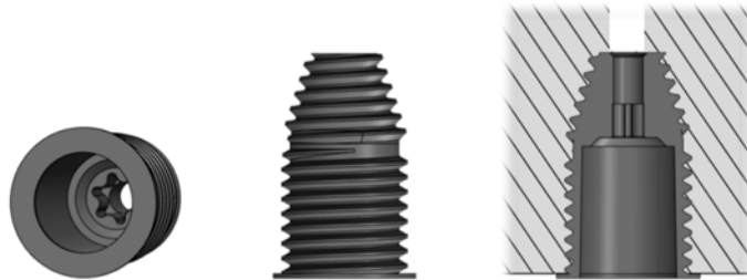
Figure 6.21: Mounting bracket 2, for recessed camera. Tapered end with self-tapping threads and a Torx screw patterned hole for installation with screwdriver.
