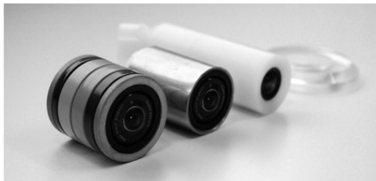
Figure 5.10: Variations of skins made for the cylinder shaped camera with an adjustable joint.
