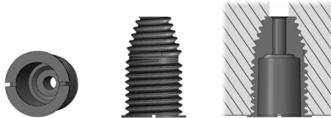
Figure 6.20: Mounting bracket 1, for recessed camera. Tapered end with self-tapping threads and a slot for installation with screwdriver.
