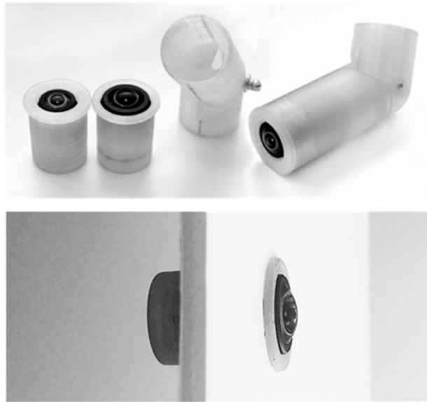
Figure 6.1: 3D-printed models of the base units and the adjustable joint.
