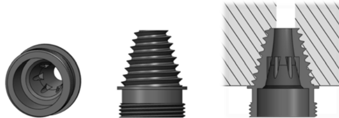
Figure 6.14: Mounting screw 2, for the adjustable camera. Tapered end with self-tapping threads and a Torx screw patterned hole for installation with screwdriver.
