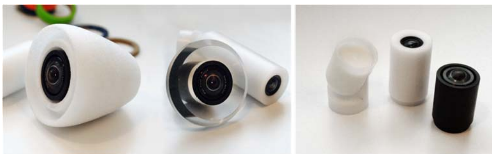
Figure 4.13: Concept models made in modelling foam and acrylic plastic.
