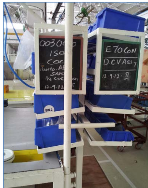
Figure 26 Material rack on wheels in position, to pick from the worktable
