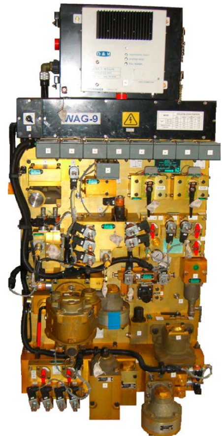
Figure 1 E70 brake panel.
