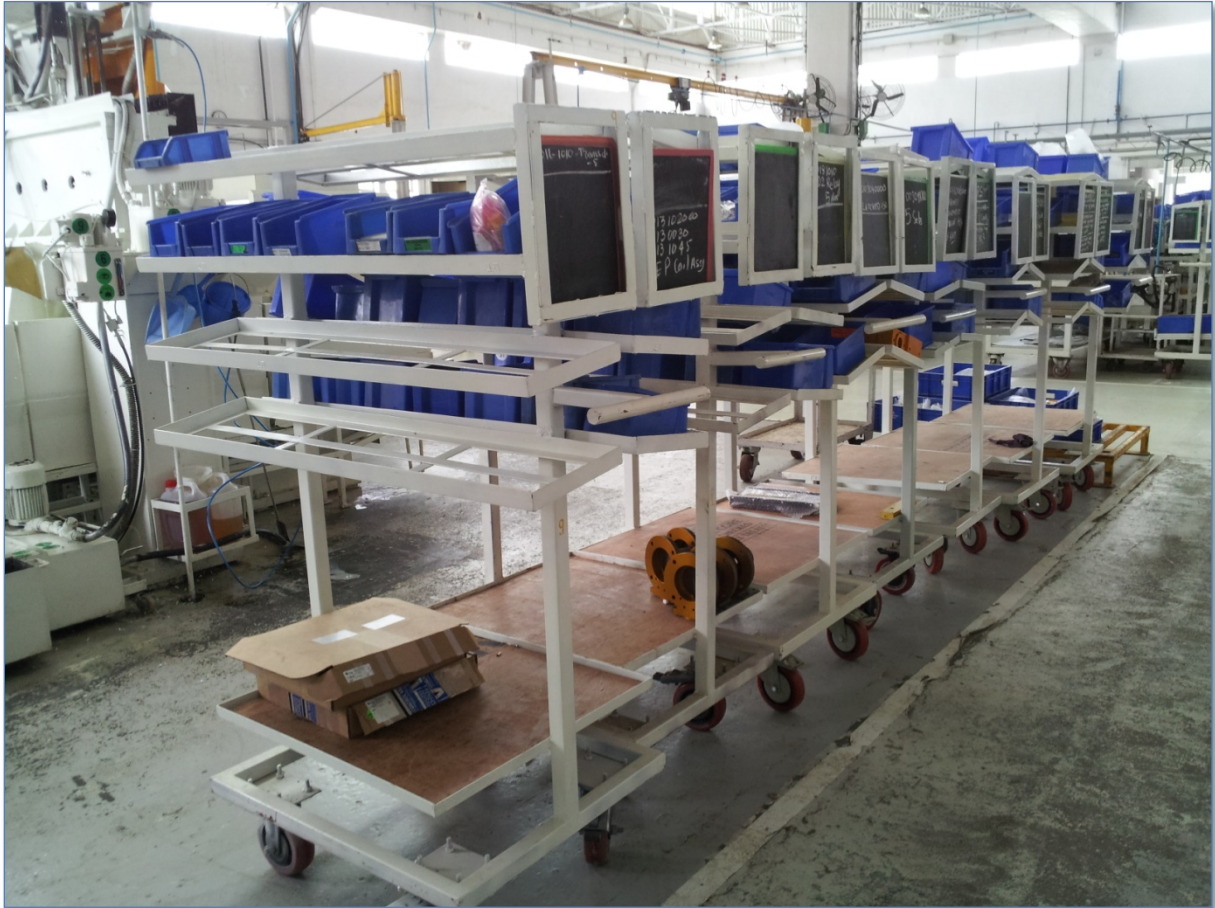
Figure 24 Material racks on wheels with "tree structure design" parked at the material market.
