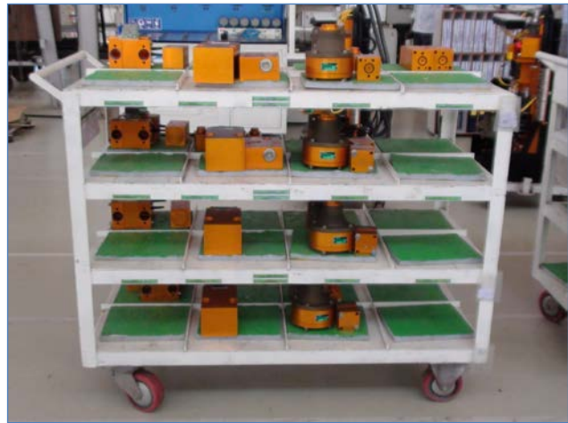
Figure 23 Plugging & sub-assembly trolley
