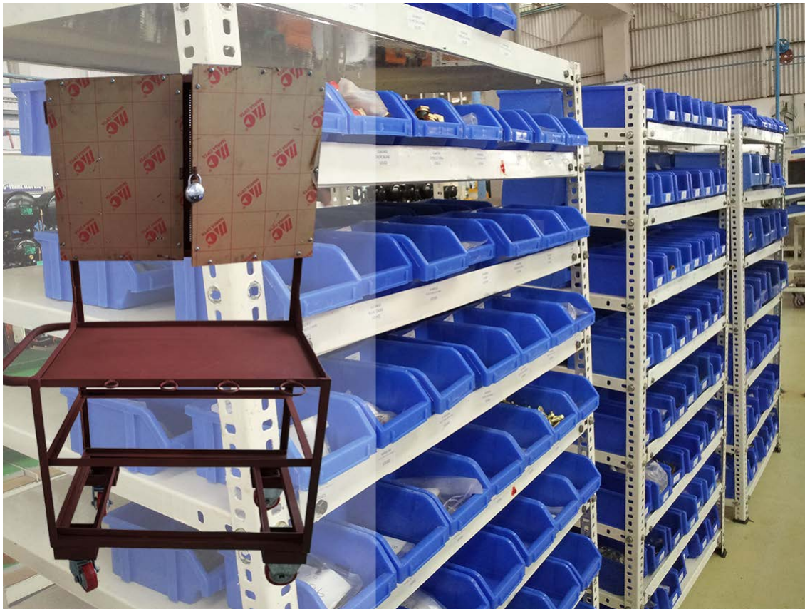
Figure 25 2 bin supermarket during the trial period & Service trolley with place for standard tools and three level assigned for c-parts picked from the supermarket.
