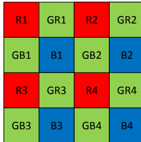
Figure 6: Schematic of the color filter array pattern.
