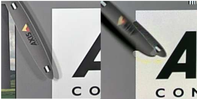
Figure 8: Picture of object rotating a 30 rpm, left: one exposure, right: multiple exposures.
