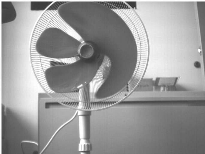
Figure 5: Picture of moving fan, shows rolling shutter effect [1].
