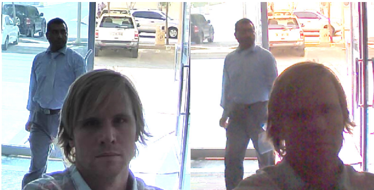
Figure 1: Left: WDR Camera, right: traditional Camera
