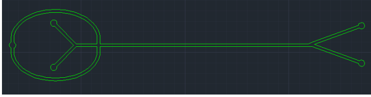
Figure 7.8: Flow focusing design for a glass channel, with a midpoint of the exit split located 1/4 of the width from the top for droplet splitting
