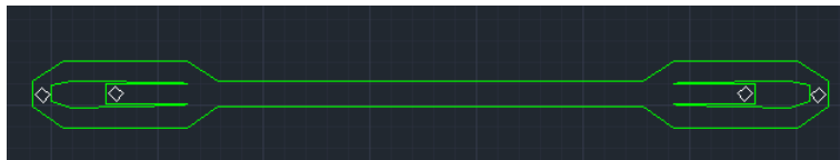
Figure 7.7: The lines in the figure shows the design of the silicon channel used in the project. The white squares shows the inlets and outlets of the channel.
