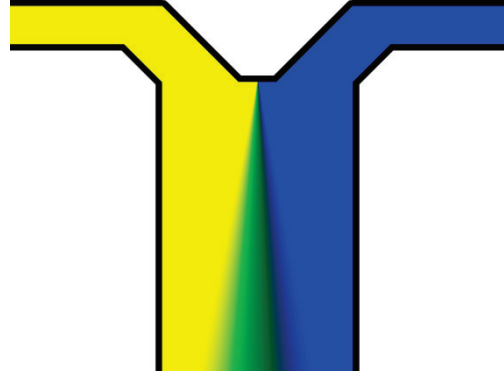
Figure 5 - The only mixing in a laminar flow is due to diffusion which here can be seen through the creation of a gradient when different fluids are led into the same channel. [a]
