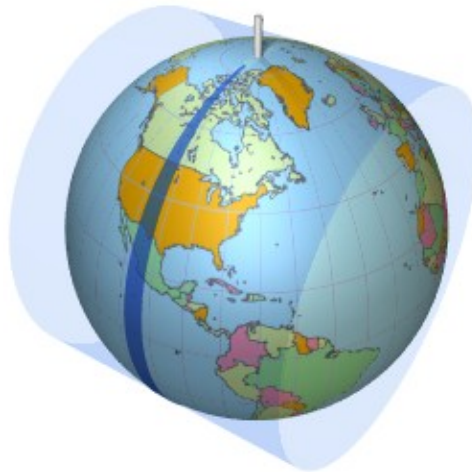
Figure 2.3: One of 60 tiles of the UTM projection. Source: www.progonos.com
