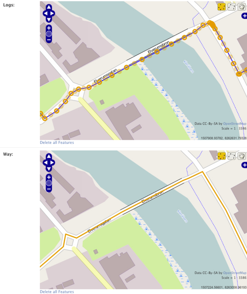
Figure 4.1: Screenshot from the logs administration tool. The top picture contains the suggested logs picked by the automated log search. The bottom picture displays the resulting route from the map matching algorithm. If the logs are missing or the algorithm has failed the logs can be manipulated by hand to achieve a satisfying result. To assist the user the data is displayed with Open Street Map as background.
