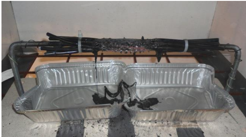
Figure 22. Extinguished cable bundle
