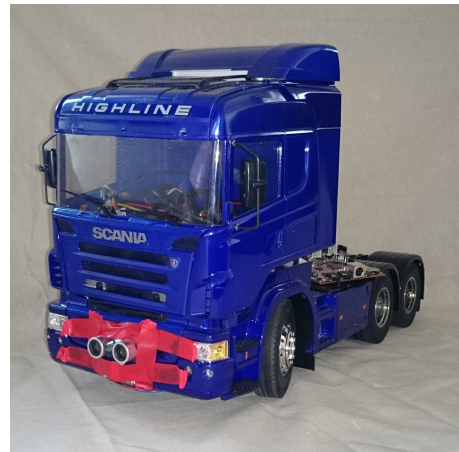
Figure 1: Fully modified RC vehicle with added sensors
