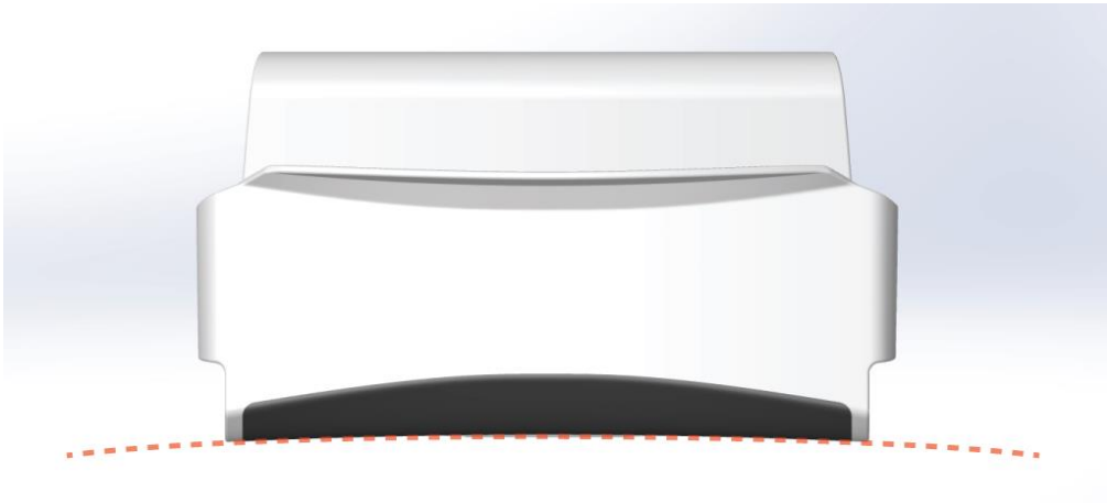
Figure 10.23 The arched bottom of the holder guides water out through the open sides of the holder
