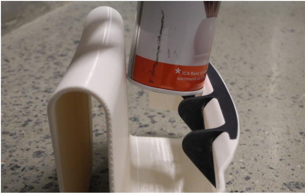
Figure 10.9 The function of the angled part of the protruding section, guiding bottles when they are placed in the holder and allowing for the front wall to flex.
