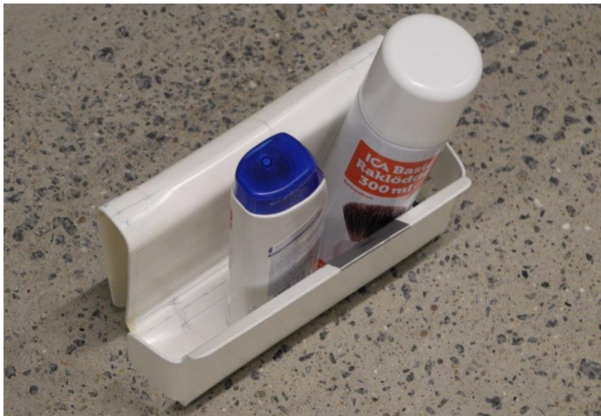
Figure 10.6 A picture of the plastic prototype, highlighting the problem of using the prototype with multiple bottles of different sizes.
