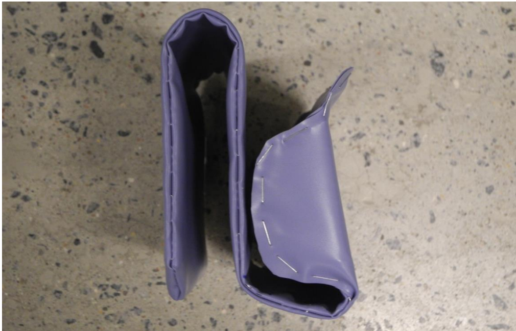
Figure 10.4 A side view of the polyurethane-coated prototype showing the tilted bottom.
