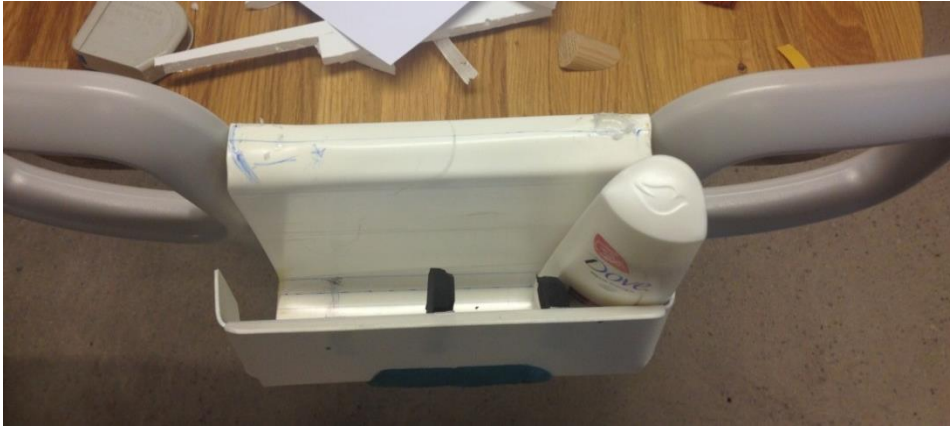
Figure 10.7 Functional prototype of flexible, separating tabs
