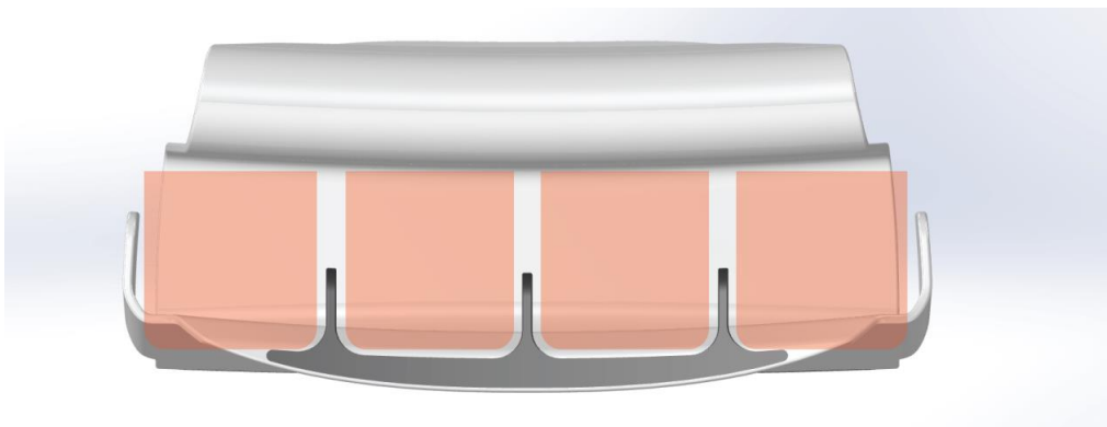
Figure 10.10 Highlights of the negative space between the tabs which constitute the four sections of the holder.
