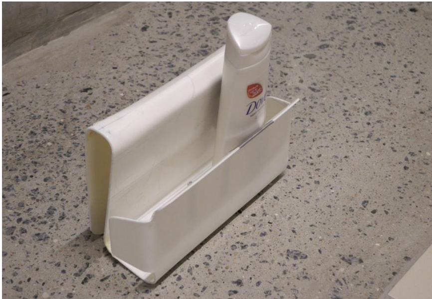
Figure 10.5 A prototype of what would become the final concept, made of a 2 mm thick plastic sheet. The prototype was made by heating up and forming the sheet.
