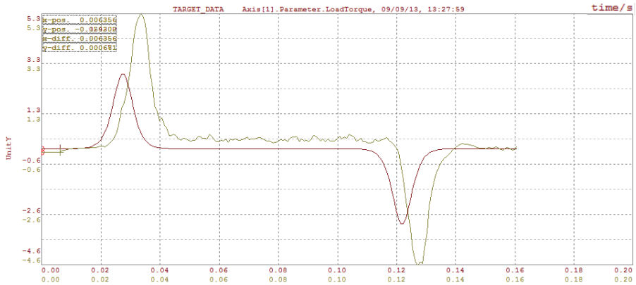
Figure 10.3 Calculated and actual torque in Nm for the first varying acceleration experiment
