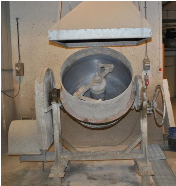
Figure 8. The concrete mixer that was used in this experiment.
