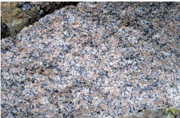
Figure 4. "Typical" granite stone: the mineral grains are very easy to see and the color of the stone is red, grey and black (Reference: SGU 2013).
