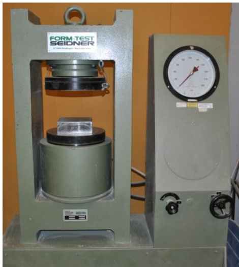
Figure 12. The compression testing machine that was used in the measurement of the compressive cube strength of the concrete cubes.
