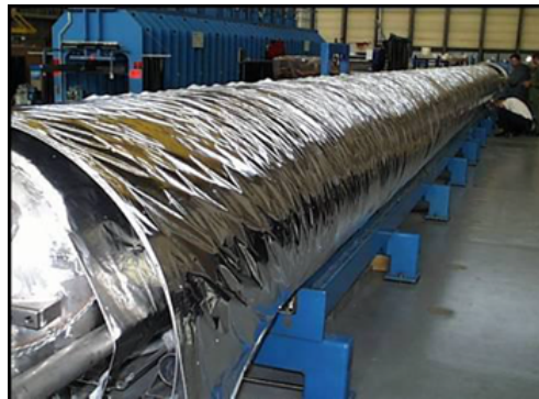
Figure 4.6 A cryostat wrapped with Multi-Layer Insulation. Source: [54].
