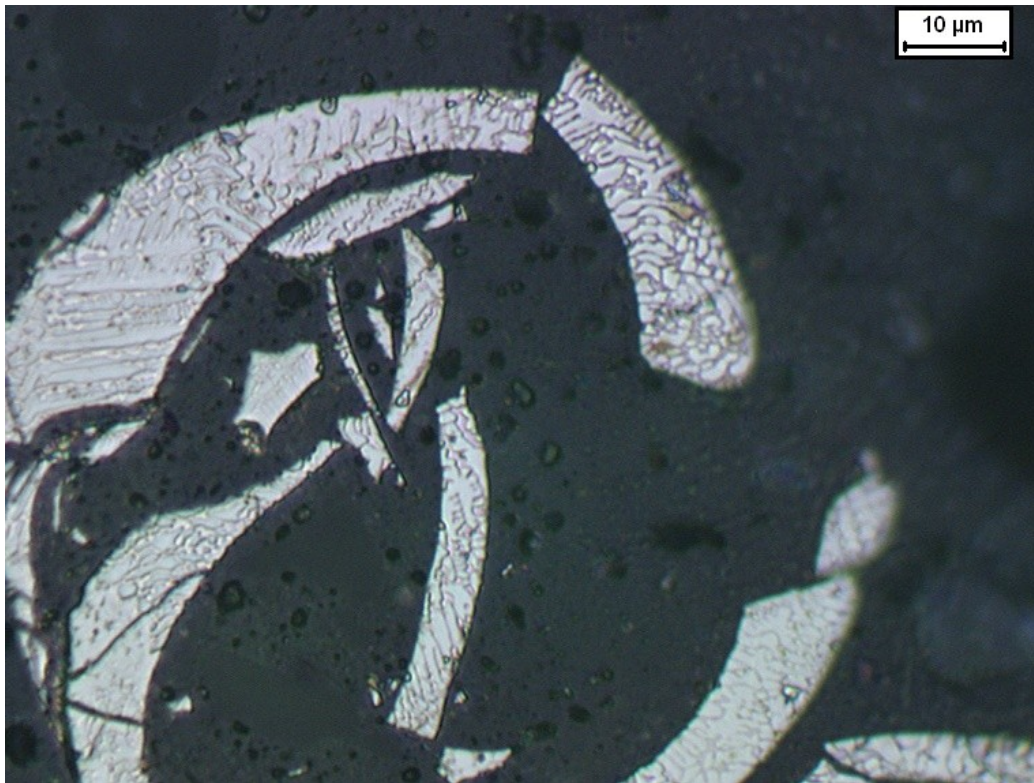
Figure 40: Example of fractured particle in the G336 material, 75-106μm.
