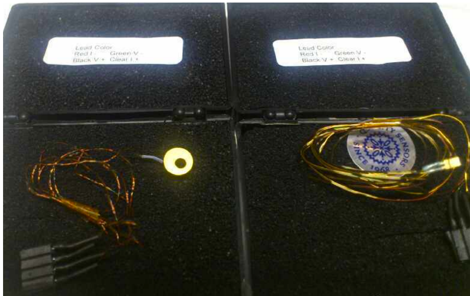
Figure 3.2. Temperature sensor in CU package (left) and temperature sensor in SD package (right). The 4-pin connector used as plug is also shown in the photo.
