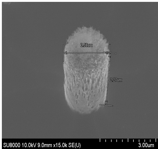
Figure 5.10 Patterned vertical Si pillar; the SEM image is taken at 30° tilt position. Mean pillar diameter is 2.48 \mu\text{m} \pm 62 \text{ nm} , the length is \sim 4.5 \mu\text{m} and pitch 7 \mu\text{m} .
