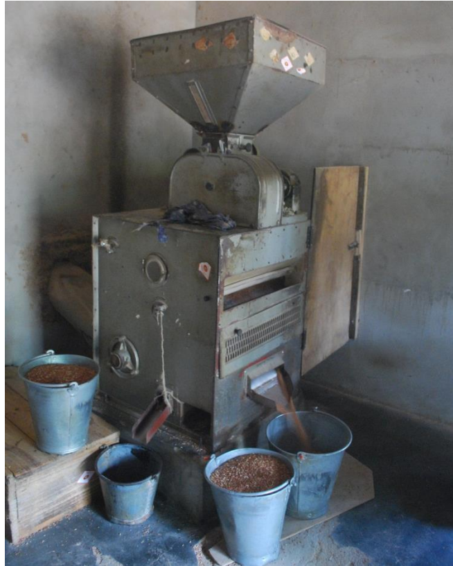
Figure 4:8. This machine is used when the husk is removed from paddy. The paddy seeds are put into the machine where the husk is removed and the rice comes out and land in a bucket, while the waste of the husk lands in another bucket, as seen in the figure. Photo: Erica Perming, 2009.
