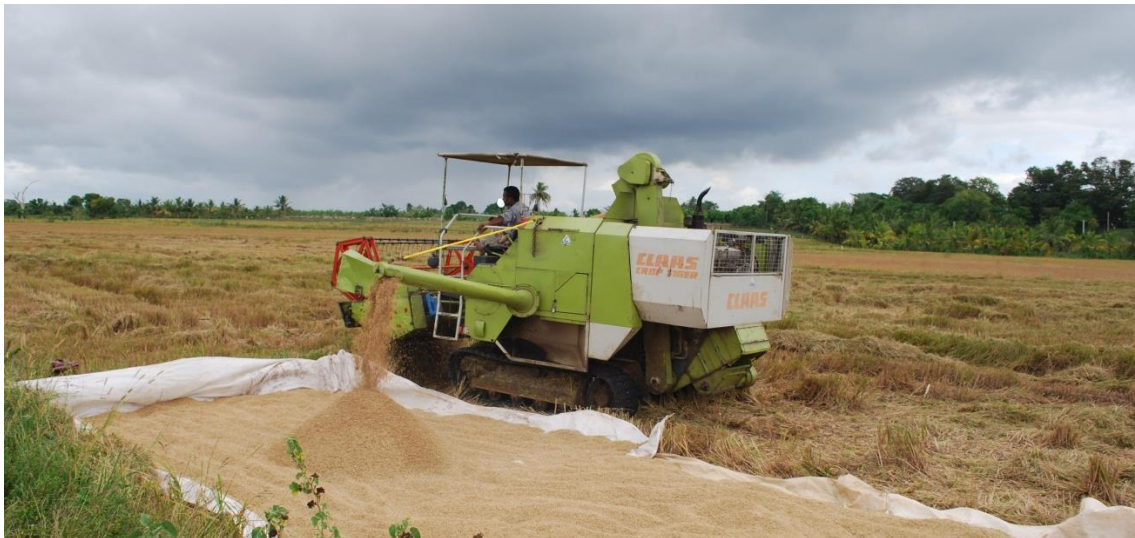
Figure 4:7. The Combined Harvester executes the whole procedure of cutting, separating paddy seeds from paddy grains and cleaning of paddy all at once. This method is used for larger fields where it is profitable to rent the machine. Photo: Erica Perming, 2009.
