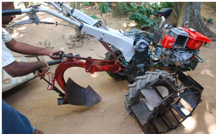
Figure 4:3. The hand tractor, also known as the land master, is used by the farmers when preparing the paddy field for cultivation. Different tools can be attached to the hand tractor and it can therefore be used when for several different purposes. Photo: Erica Perming, 2009.
