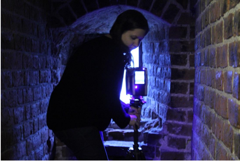
Figure 18. Picture from the acquisition with 3D laser scanner, I'm placing the laser scanner in the narrow window niche (photo taken by: Nicolo Dell'Unto).
