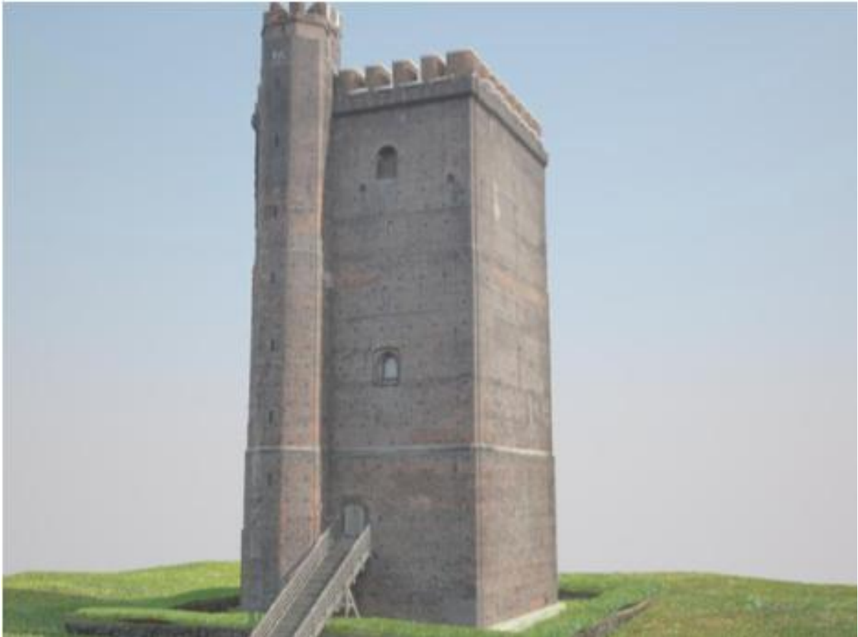
Figure 1. A screen capture of a 3D model of Kärnan. The model was mainly reconstructed with Image based modeling, however the stairs and the roof of the tower needed to be modeled from pictures (Holmqvist, Moulin & Roe, Group work in Master's Programme: Archaeology – Theory and practice).
