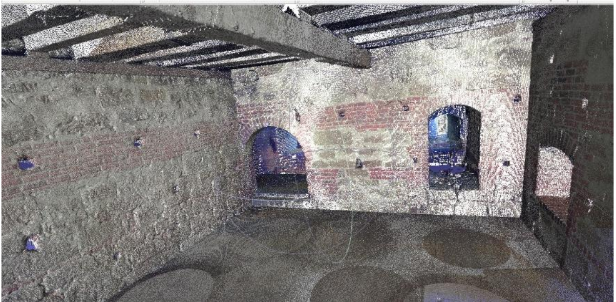
Figure 19. Screen capture of the merged point-cloud of the second floor in Kärnan, in Meshlab.
