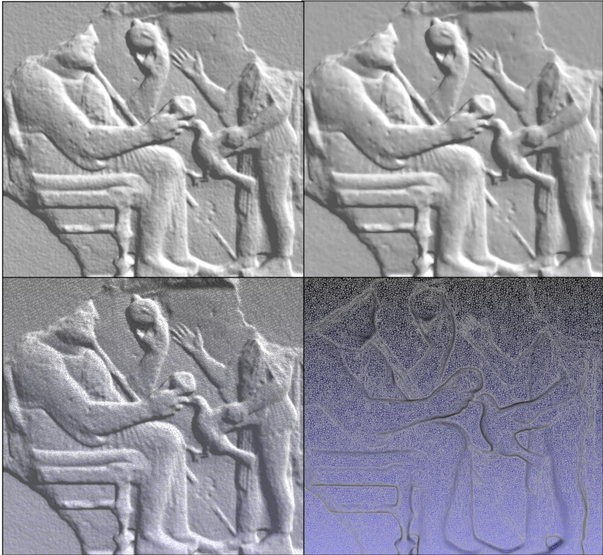
Fig. 8 A comparison of one of the panels before (left) when it contained 458, 841 faces, and after (right) the use of the quadratic edge collapse tool when the face count was reduced to 100,000. The top two images show the surface of the model. Notice that the surface of the post quadratic edge collapse model looks blurry and that some of the smaller details have become harder to see or have disappeared - especially the folds in the clothing. The bottom images show the wireframes of the corresponding images above (when viewing a wireframe only the edges of the faces are visible). All images were made using the 'Snapshot' tool in Meshlab and for each image I chose to leave the background color on because in the case of the wireframe images it shows what a difference the quadratic edge collapse can make. Due to the high face count, the wireframe on the left is so dense that the blue and black background color is not visible, while on the right image with the lower face count the background is clearly seen.
