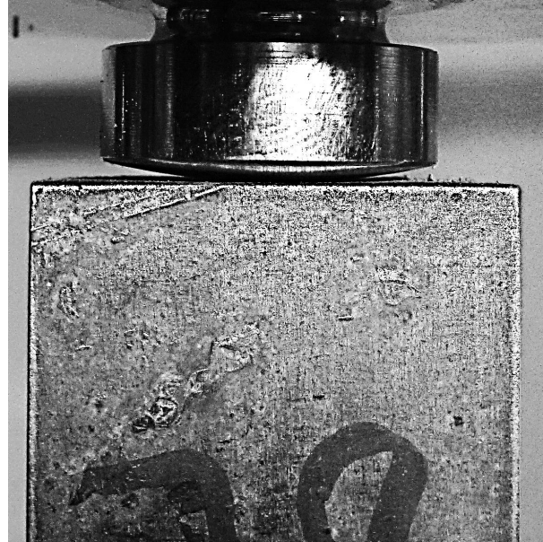
Figure 5.5 Upper connecting surface (pinned at high loads)
