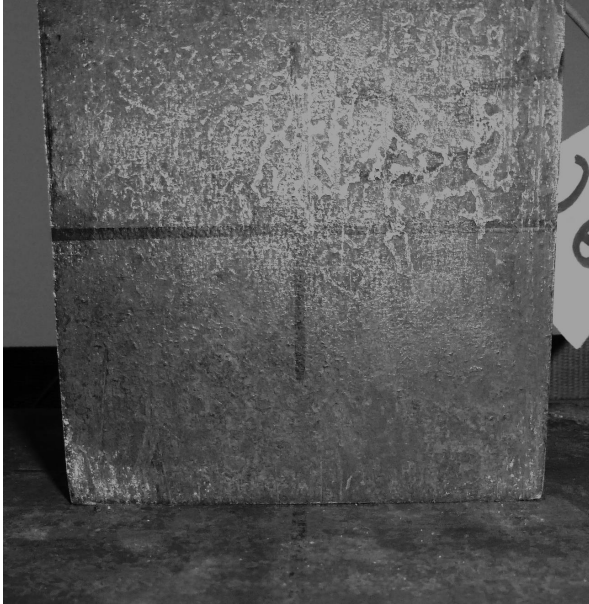
Figure 5.4 Lower connecting surface (fixed at high loads)
