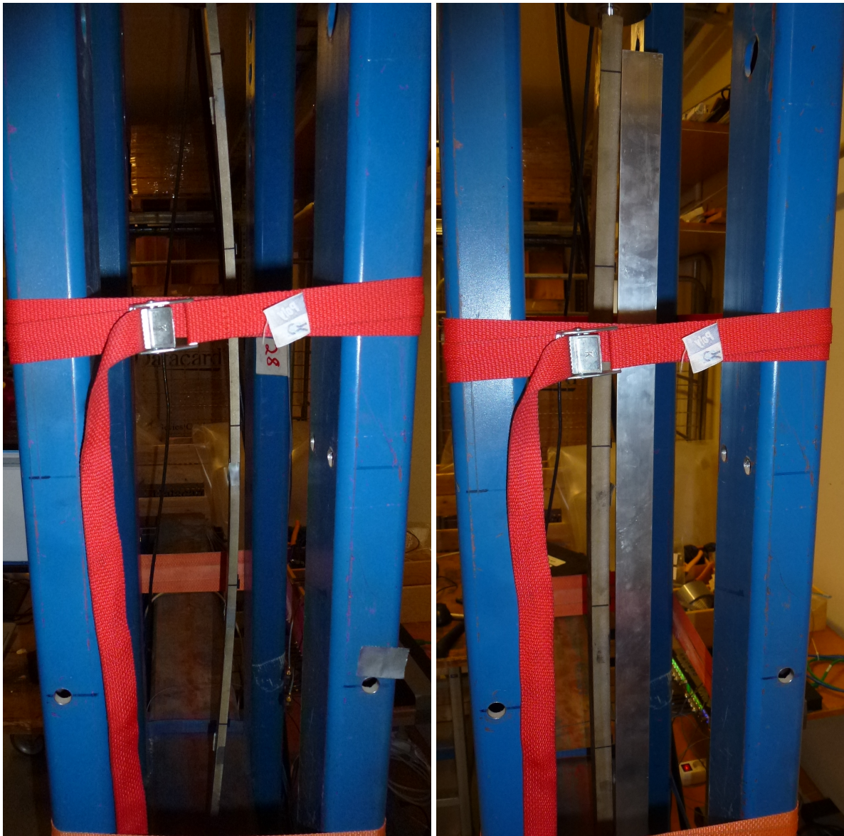
Figure 5.7 Deformation of the beams at highest loading level (left: B1020 right: B2040 with reference ruler)
