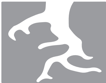
Figure 2.6 The structure of the pores in activated carbon. The surface in which the ions can fold on is much wider than in a traditional capacitor.
