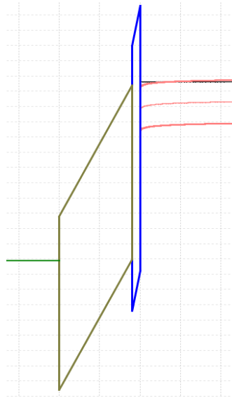
Figure 24: Under positive applied bias electrons are injecting from substrate to high-k.
