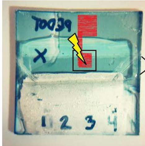
Figure 2.4. The solar cell device structure Glass/ITO/PFPA-1/polymer:fullerene/PEDOT:PSS(PH1000)/Glue/Glass. The yellow arrow marks the site of excitation, red area – ITO contact.
