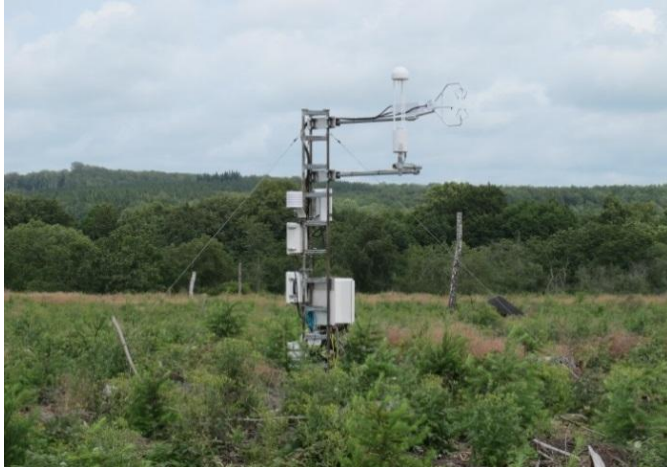
Figure 4. Eddy-covariance tower at the clear-cut 2011. Measurements of carbon balance were carried out during 30 May - 27 August 2013.
