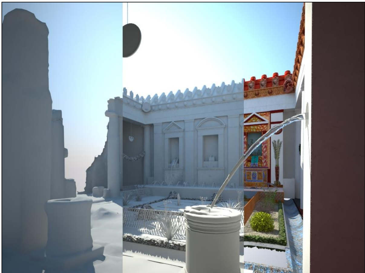
Fig. 02. Workflow of the modelling: mesh realized after the acquisition campaign (left), modelled geometry (middle) and geometry complete with the textures (right) (M. Perlińska).
