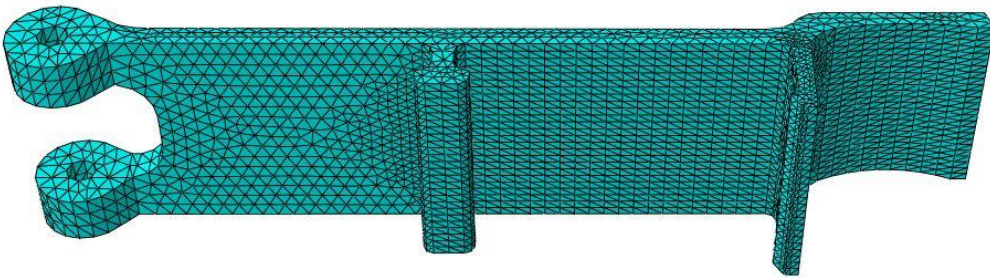
Figure 4-8. Mesh at the back of the hatch
