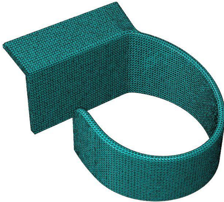
Figure 10-5. Global mesh size of 0.7 mm.
