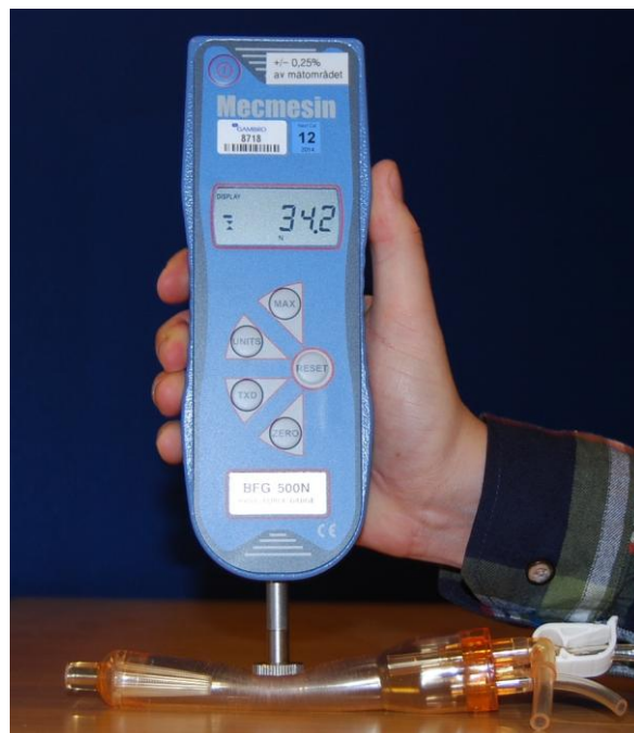
Figure 10-1. Test of the elastic modulus of the chamber.
