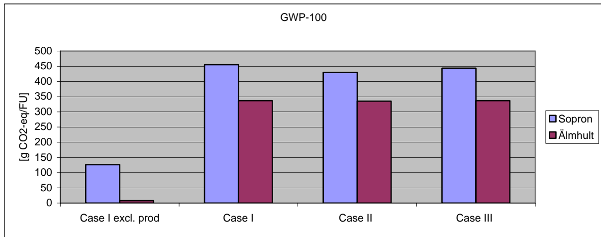
Figure 21. Total GWP-100 caused by Swedwood activities (mixing process and transport), when excluding the mixing process of water-borne lacquers in Case I
