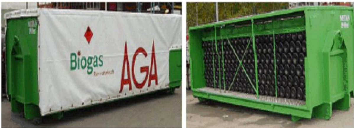
Figure 22 To the left; a mobile CBG storage with a fireproofed cover and to the right; gas bottles arranged in the storage. (Schröder, 2008)
