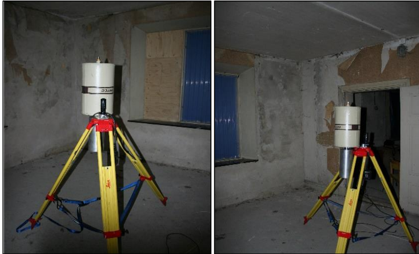
Figure 8: HPGe detector positioned in the center of the corner room of the house, and images showing the HPGe detector facing the corner towards the fallout area ( left frame ); the HPGe detector facing the short side of the room with a window ( right frame ). Note that the cryostat is mounted above detector to minimize shielding of ground emitted photons.
