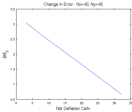
Figure 3.53: Change in error between exact and approximated solution of Eq. 3.6, N_x = 40, N_y = 40 , with constant ansatz functions and M_x = M_y = 3, 4, 5, 8, 16, 32 .
