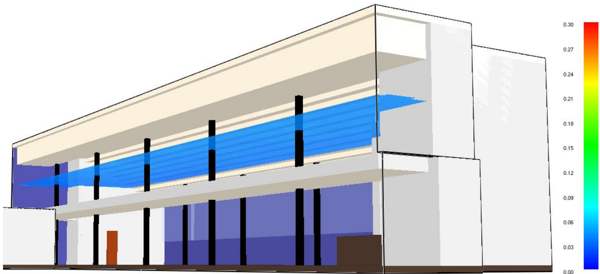
Figure 4.7 FIC level at 1.6m high from the balcony for the Bookcase fire (at 270s)
