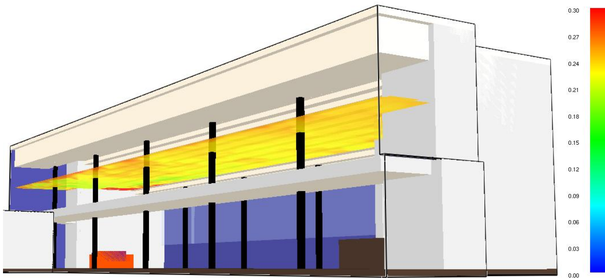
Figure 4.6 FIC level at 1.6m high from the balcony for the Sofa fire (at 270s)
