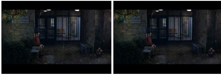
Figure 4.30: The figure to the left shows the original scene. The figure to the right shows the scene with reduced precipitation. The restoration algorithm for removing the precipitation is subtraction. This scene contains light amount of precipitation
