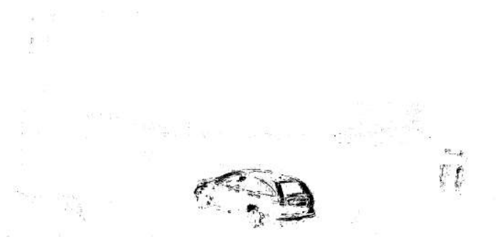
Figure 4.11: The result from the chromatic algorithm which has been compared to the mask in 4.2. A threshold of 16 is used.
