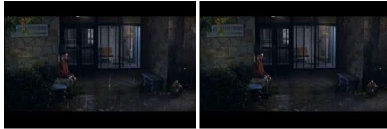
Figure 4.27: The figure to the left shows the original scene. The scene to the right shows the scene with reduced precipitation. The precipitation is removed by taking the mean of three images. This scene contains light amount of precipitation.
