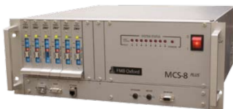
Figure 2.5 The MCS-8 – the control system that comes with the FMB Oxford robot.
