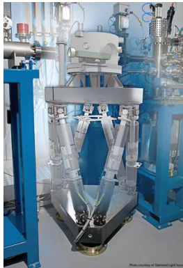
Figure 1.1 Example of monochromator on Stewart Platform
