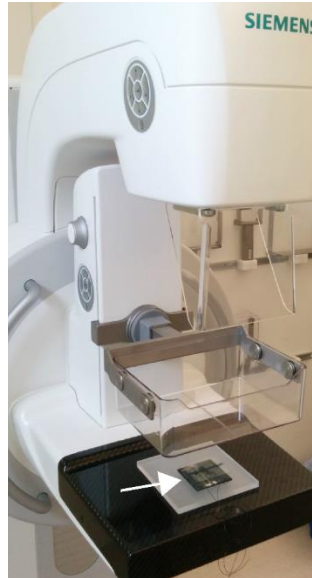
Figure 28. Siemens MAMMOMAT machine taking an x-ray image of the sensor. The white arrow shows the sensor.
