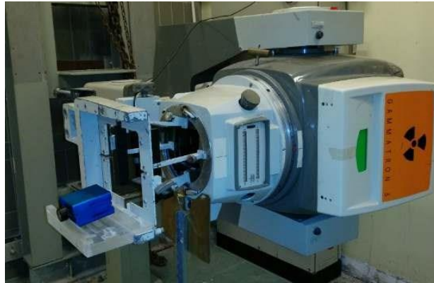
Figure 29. The Gammatron 3, used for radiation tests.
