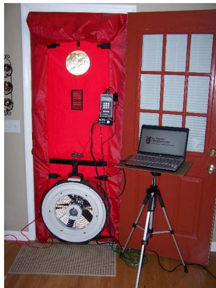
Figur 4-2 Blower door. (Bankvall, 2013)
