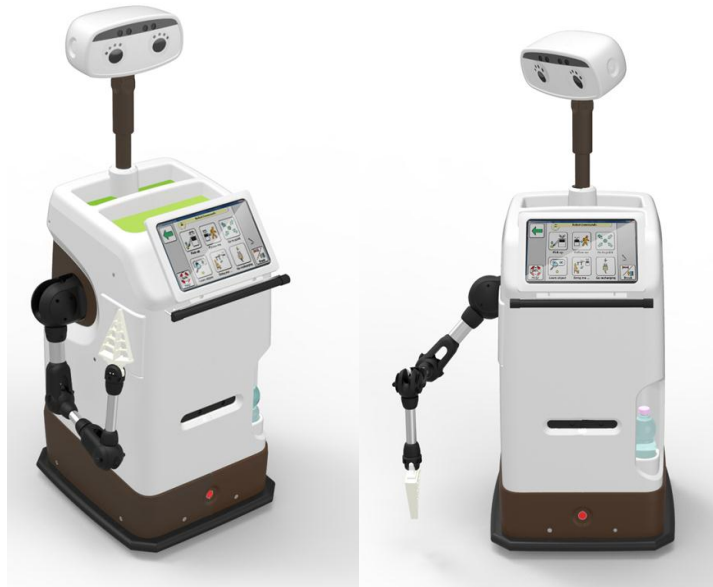
Figure 4: Latest model of the HOBBIT robot [6]
