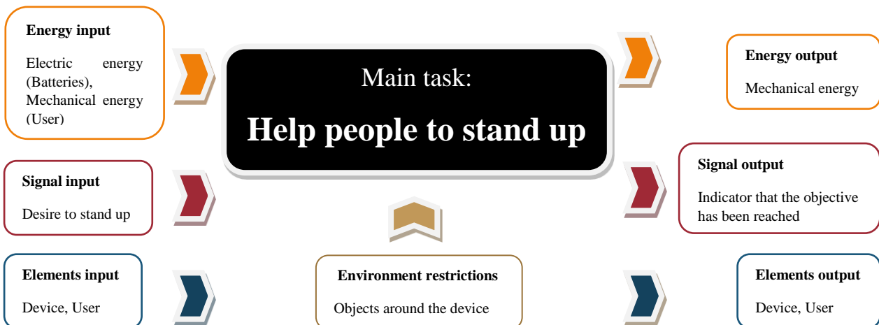
Figure 14: Black Box diagram to define inputs and outputs of the process the device should complete
