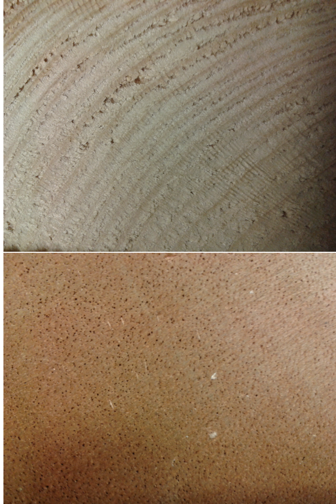
Figure 4.3: Picture of the cross section from a pine sample (top) and from a mahogany sample (bottom). The two wood samples show completely different structures.
