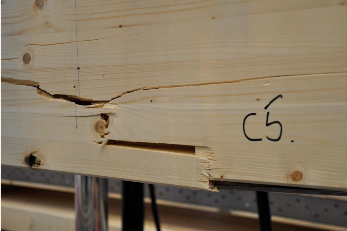
Figur 6.61- Balk C5, dragbrott i fingerskarv.
