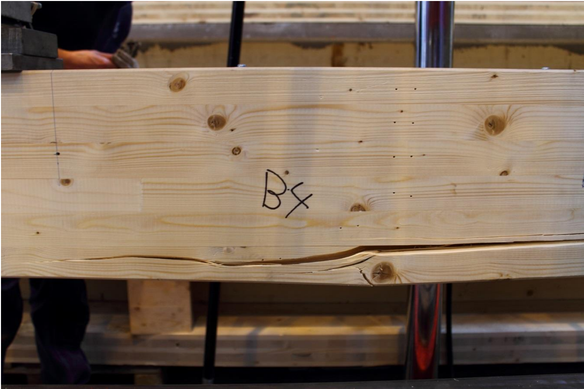
Figur 6.47- Balk B4, dragbrott runt kvist.
