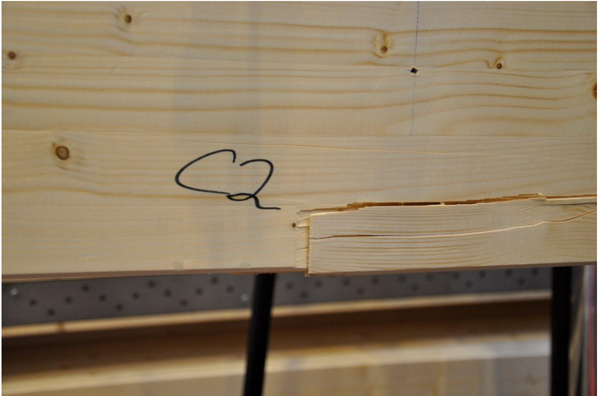
Figur 6.55- Balk C2, dragbrott i fingerskarv.
