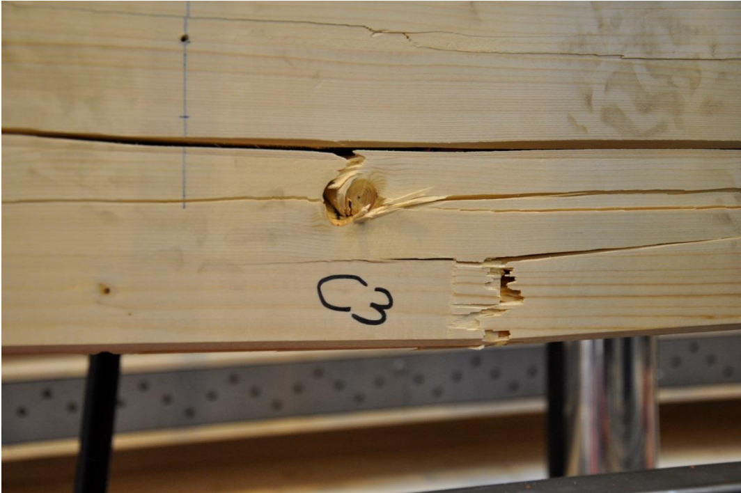
Figur 6.57- Balk C3, dragbrott i fingerskarv.
