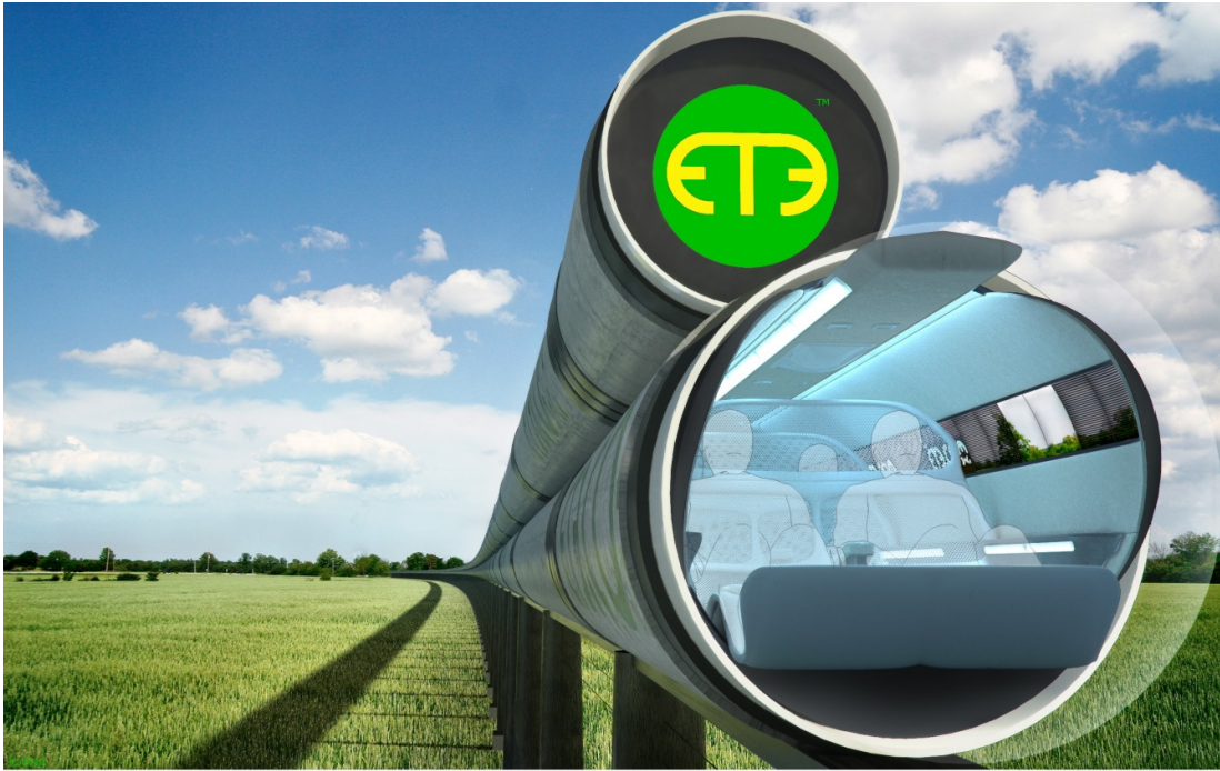
Figure 7. ET3 cut through image; circular cross section (Image: Visualization by ET3).
