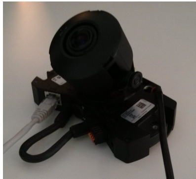
Figure 2.5 The Axis P3367 camera, without its dome casing
