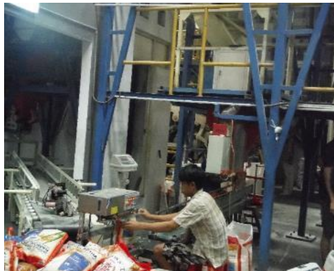
Figure 4. Filling machine and manual sealing of 5kg rice in plastic bag
