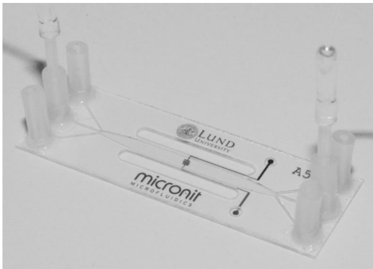
Figure 5.4. Image of the glass chip. The two circular metal areas to the right of the middle are the connection sites to the electrodes (electrode pads). One can be contacted from the top side of the chip and the other from the opposite side. In the middle of the channel the electrodes can be seen. At the right and left sides of the chip the three inlet and three outlet tubing are glued to the chip.
