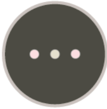
Figure 4.6: Probe 2 with three fibres for possible source-detector separations 1 mm and 2 mm.
