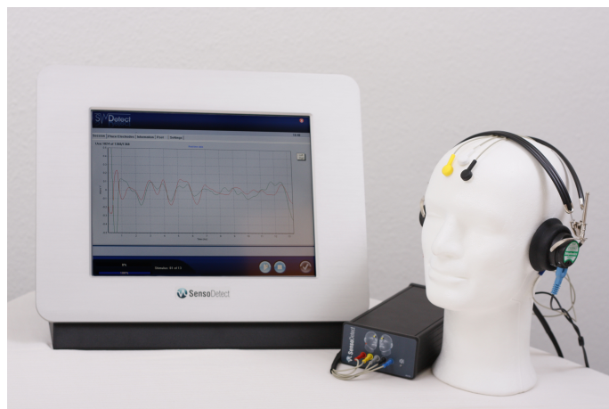
Figure 6: The BERA-equipment setup. The frontal electrodes of the two channels, left in black and right in yellow, are here seen. The corresponding opposite pole of each are located right behind each ear. The channels are attached to ground separately. The AD-conversion is performed with a resolution of 0,05 mV using 16-bit hexadecimal conversion. Image source: [59].
