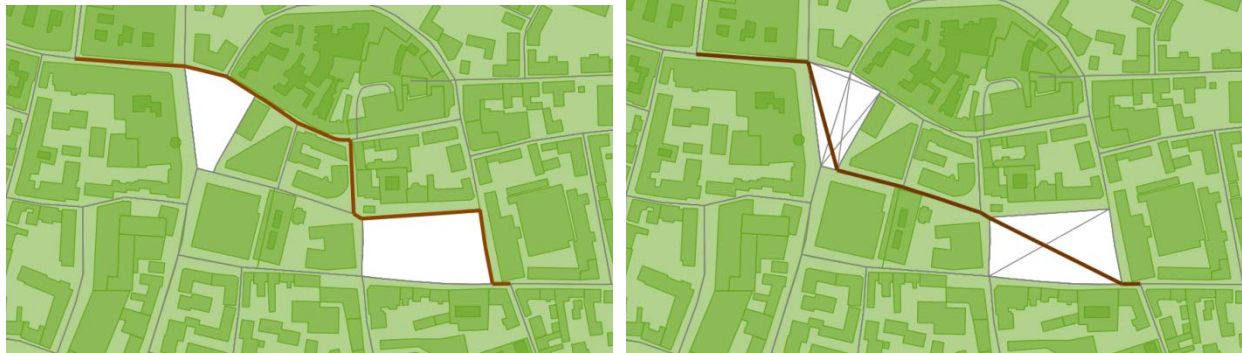
a. b. Figure 6.8. a. The routing result based on original data from OSM using Dijkstra algorithm from pgRouting, b. The Dijkstra routing result based on road network data with added paths in opens.
