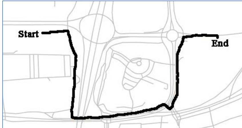
Figure 5.5. Screenshot of shortest route result with weighted cost. (NOTE: Successful routing result is illustrated, as it chooses the cheapest path by excluding motorways, and using pedestrian paths instead).
