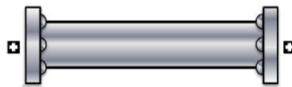
Figure 61: Ideal pipe Simulink icon. It can be connected to the different components that share the same type of connectors.
