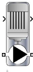
Figure 70: Pump Simulink icon. It can be connected to different components and it includes one input for a heat source and an output for plotting data in case of using a scope.
