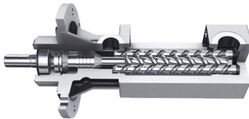
Figure 7: Screw pump inside. The case holds the screws that moves the fluid along them increasing its pressure. The axe torque is generated by a brushless DC motor. (Source: http://www.knoll-mb.de/ ).
