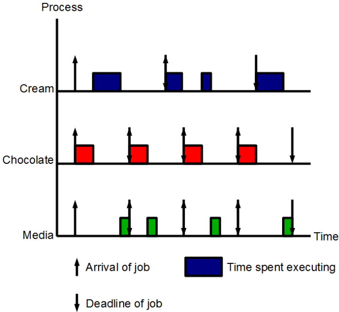
Figure 2.5 An example of three processes executing on the same processor, assured at the criticality of the media process.
