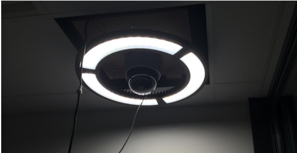
Figure 9.5 The Philips luminaire modified to a test rig with a P55 camera installed
