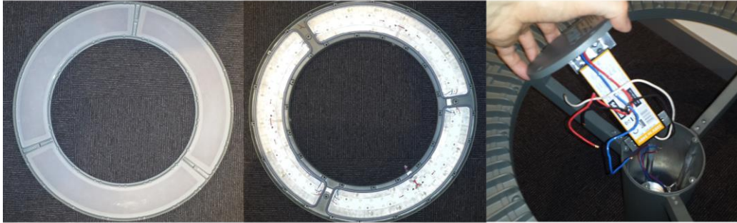
Figure 9.2 Left: The bottom plate of the construction. Center: Top plate of the construction. Right: The cylinder construction containing the driver.
