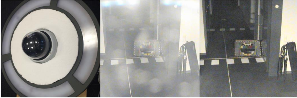
Figure 9.7 Left: The test rig prepared with a Styrofoam brim. Center: Picture without the brim. Right: Picture with the brim
