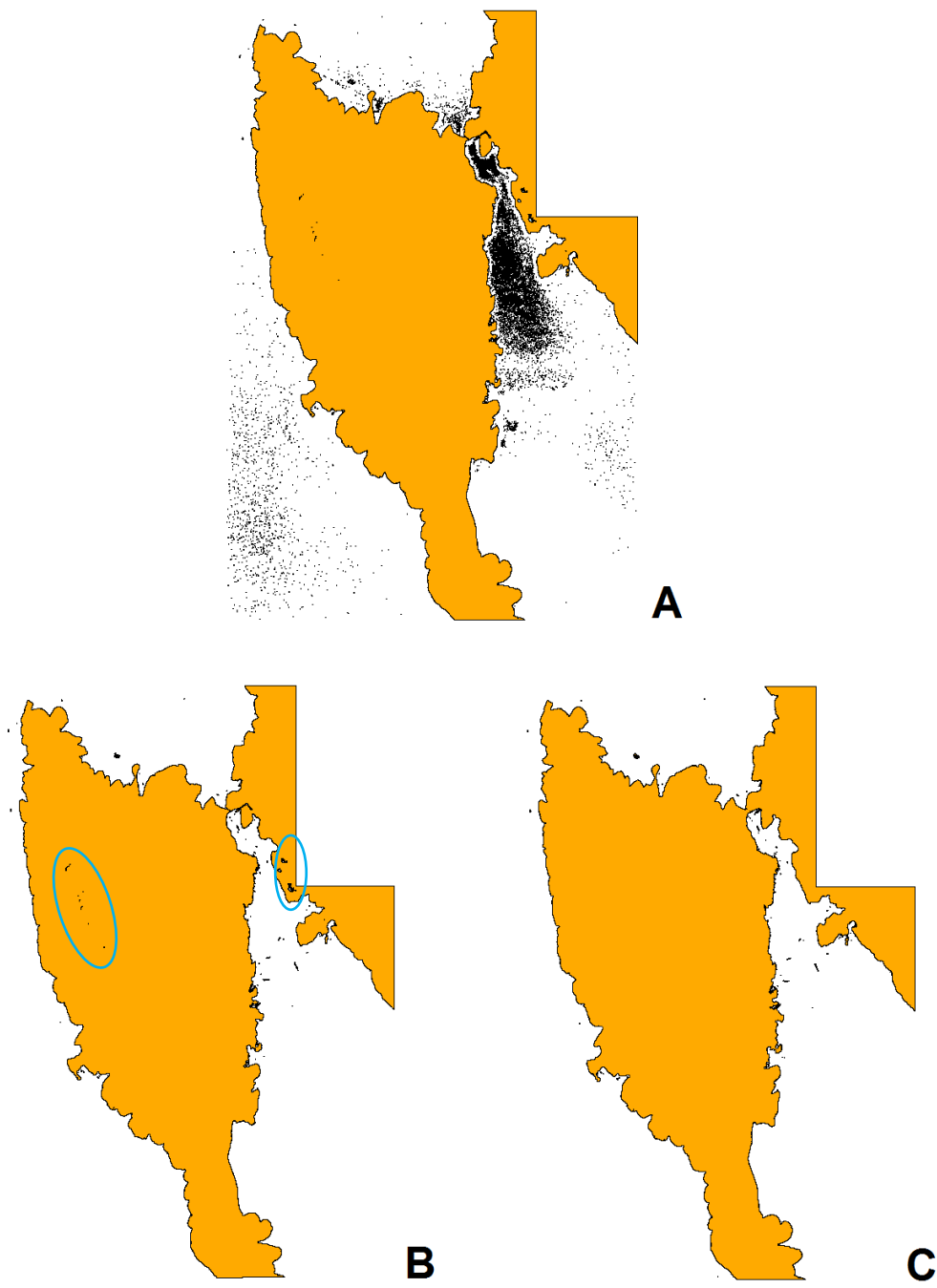
Figure 3.3) raster threshold mask converted to shapefile (A), and then manually edited to remove isolated water pixels that incorrectly categorized as land (B) and the final result after applying union, eliminate and dissolve operations orderly (C).
