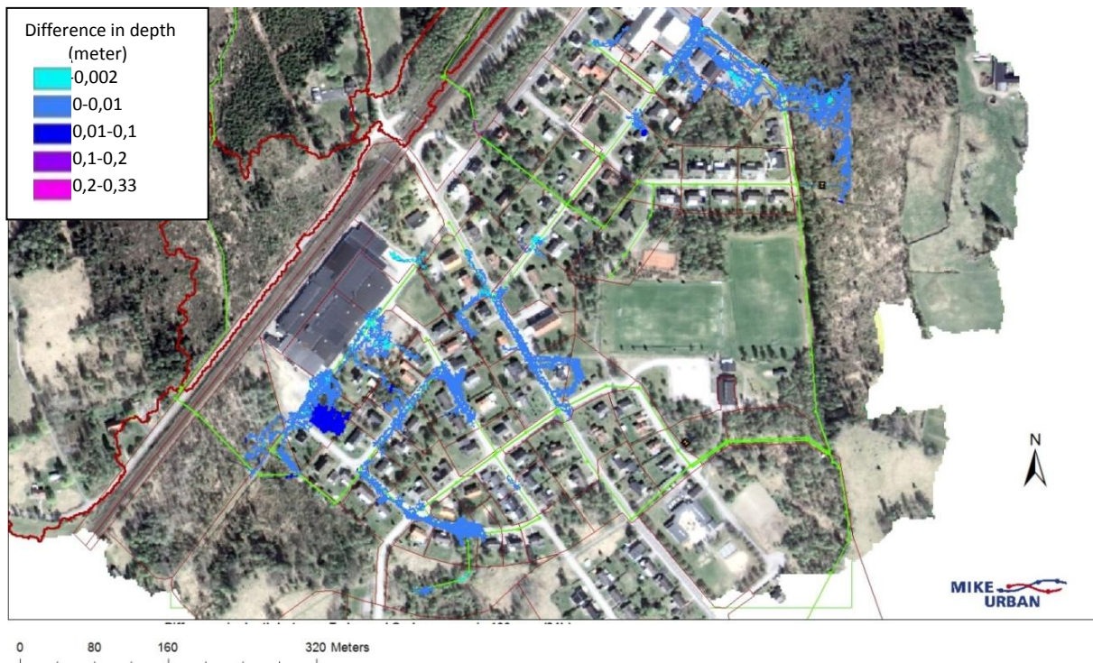
Figure 15: The difference in depth between the climate scenarios Today and Carbon storage , visualized through subtracting the projected maximal flooded extent in Carbon storage from Today . The simulations are made using a precipitation of 100-year recurrence interval (24-hour) with a MIKE FLOOD model over Eneyrda.
