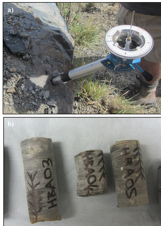
Fig. 9. a) The orientation sleeve equipped with a sun compass, a magnetic compass and inclinometer. b) Core samples were marked in order to specify the direction of drilling.
