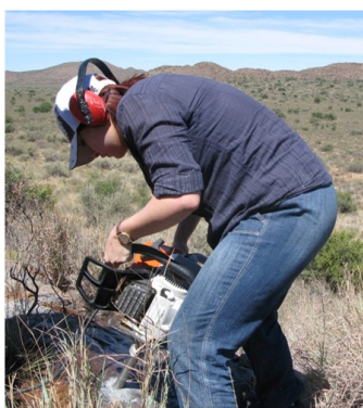
Fig. 6. All samples were drilled using a water-cooled portable drill.
